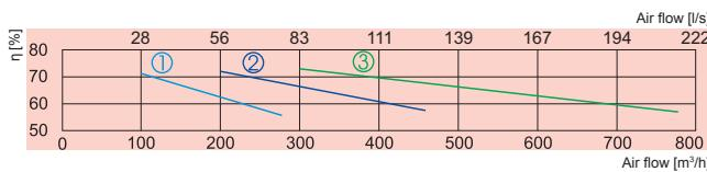
Calculated temperature efficiency (balanced mass flow) EN 13141-7:
