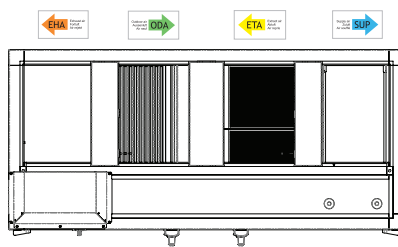
View from inspection side
