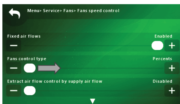
Fig. 20 Fans speed control 1
